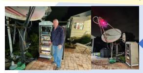
Tony KC6QHP — 02/20/2024 10:11 PM — Tonight I visited the QTH of K6QPV - Greg Bailey in San Diego. This is his 10 GHz EME station. The outdoor enclosure contains a 250 watt TWT amplifier!! Flexible Waveguide connects the amplifier output to the dish feed. Dish is 2m diameter
