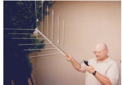
The operator keeps an eye on the signal strength while using the antenna, noting azimuth, elevation and polarity
