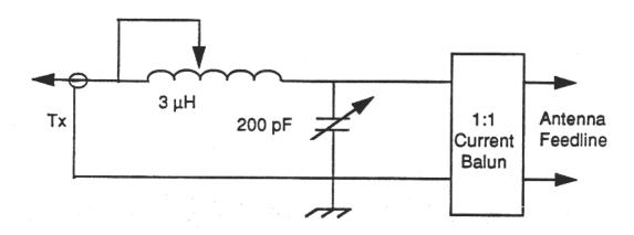
The balun is a Jerry Sevick design with a 100 ohm impedance winding.
