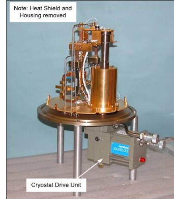
Ka-band (32 GHz) low noise amplifier
