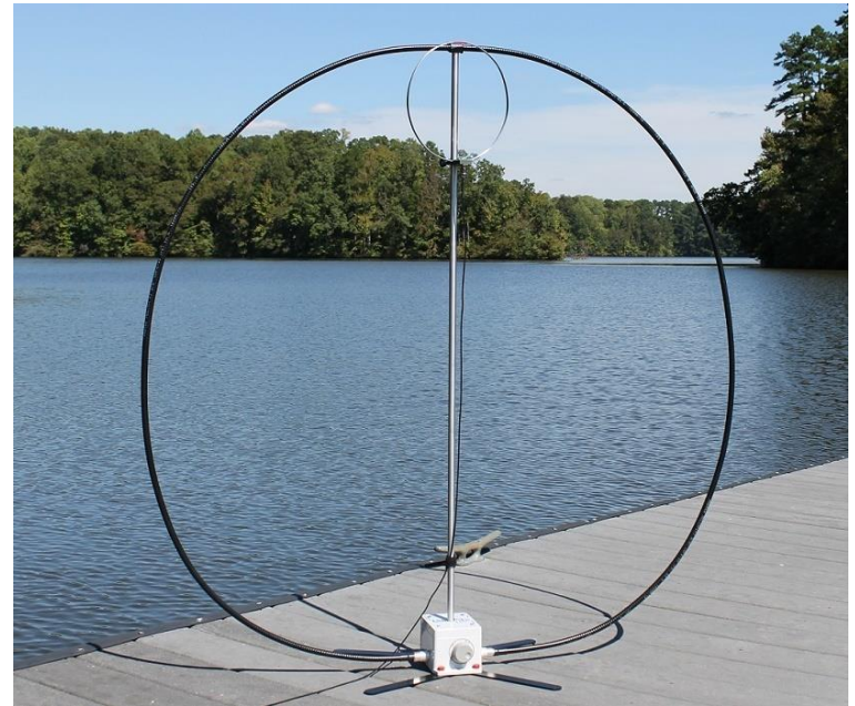
W4OP 48" Loop (LNR) is more efficient on 40M than the common 36" loops
